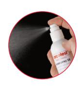
The surface tension is determined by spraying test ink onto the surfaces to be assessed.
